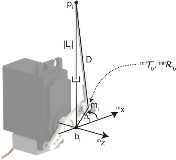
Fig. 5. Local coordinate system of a particular servo motor ( $i$ ) ( $i$  even) with indication of variables and constants involved in the computation of the length of a virtual leg  $L_i$ .
