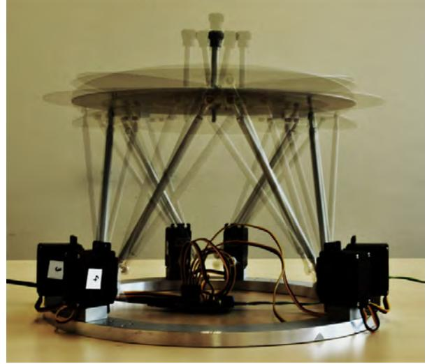
Fig. 6. Photograph of the low-cost Stewart platform overlaid with a series of images indicating the range of platform's motion.
