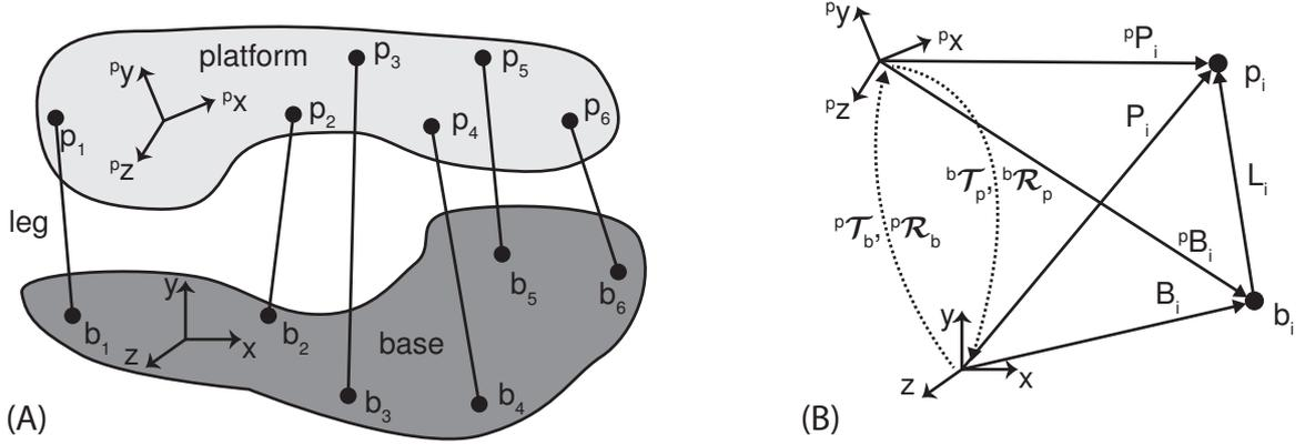
Fig. 3. Schematic illustration of a SP indicating the mathematical notation used throughout this work. (A) shows the upper platform and the lower base with their corresponding coordinate systems and the attachment points of the legs (after [2]). (B) shows the transformations between and the vector notation in the two coordinate systems.
