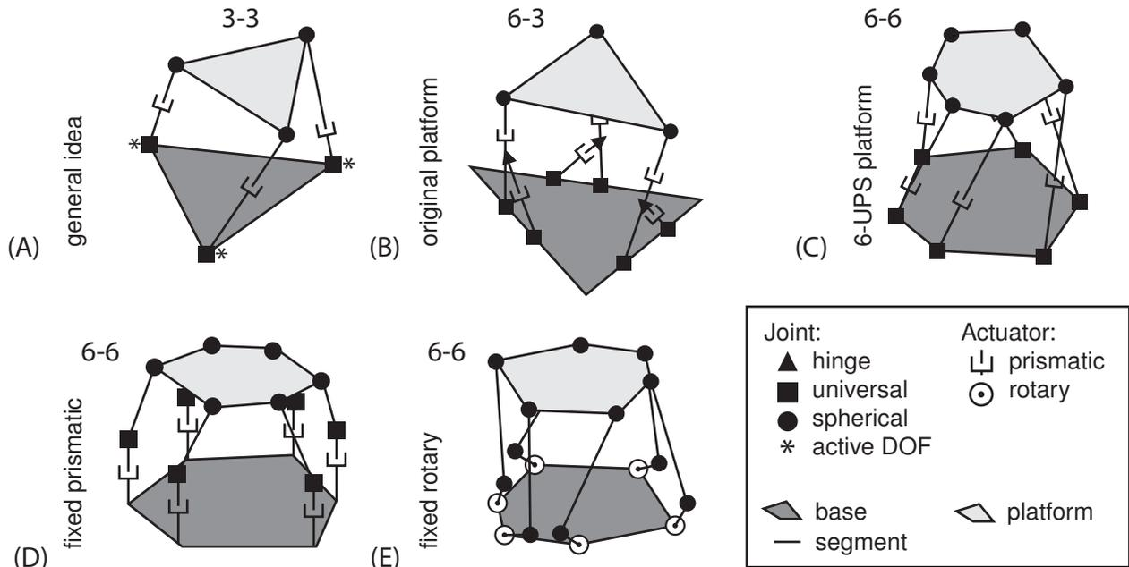
Fig. 2. Simplified depictions of several GSP architectures. (A) the original idea by Stewart and (B) its actual realization with 6 prismatic (hydraulic) actuators [1]. (C) the most typical realization of a 6 DOF platform commonly known as 'the Stewart platform' or a hexapod robot. (D) and (E) show examples of Stewart platforms with, respectively, prismatic and rotary actuators fixed at their bases. The latter platform is further elaborated on in this work.
