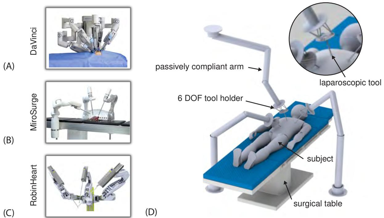
Fig. 1. Robotic minimally invasive surgical systems including (A) the commercially available DaVinci [19] telerobotic system and a selection of research projects: (B) the MiroSurge [20] of DLR (Germany) and (C) the RobinHeart  $mc^2$  [21] of the Foundation for Cardiac Surgery Development (Poland). (D) is the conception of a surgical robot consisting of passively positionable arms and 6 DOF platforms for holding and adjusting the positions of laparoscopic tools.
