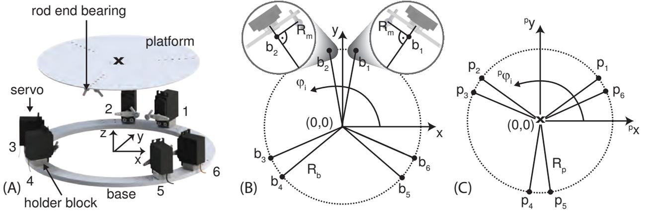
Fig. 4. Exemplary SP design with fixed rotary actuators. (A) is the isometric view of the arrangement of servo motors; connecting rods are not shown for the sake of clarity. (B) and (C) show the geometrical arrangement of leg attachment points in agreement with the notation from Fig. 3. Platform's origin is marked with an  $x$ .
