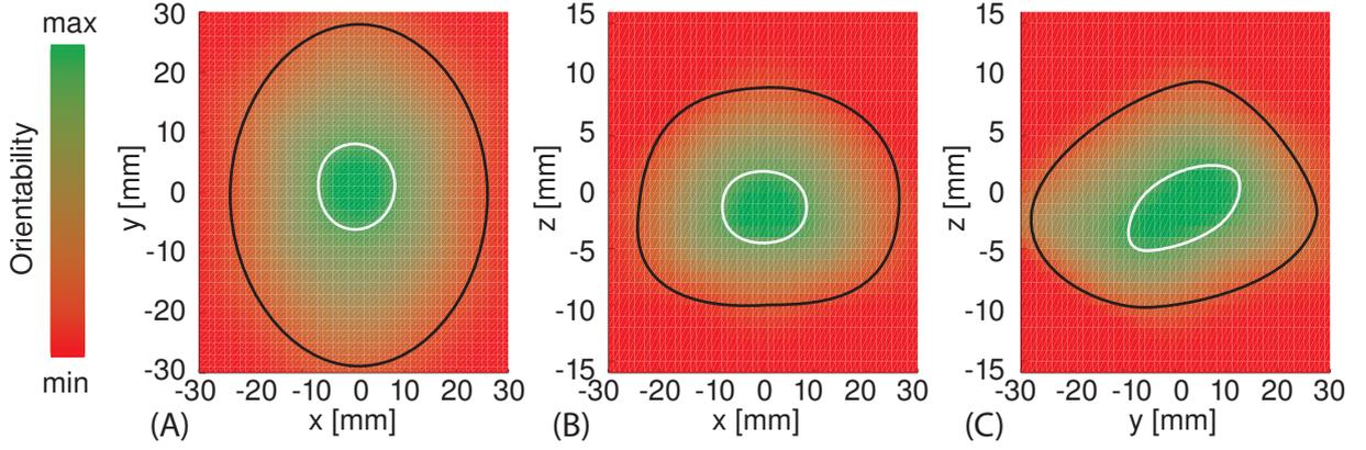
Fig. 7. Diagrams illustrating the work area of the low cost platform. Any position within the regions encircled by a black curve can be attained. Color-coded is the ability of the platform to change its orientation at a given location. Regions encircled by white curves allow the platform to change its orientation most freely.
